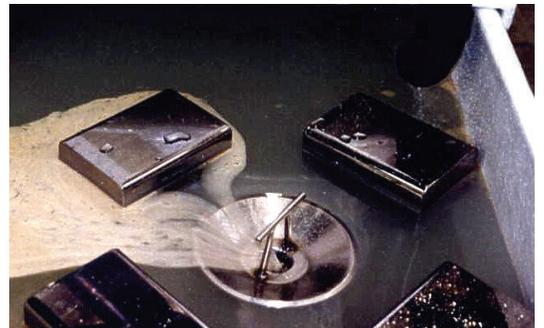
Using the appropriate weir setting, Megator skimmers will deal equally well with thin surface layers of light oil or concentration of heavy oils.
